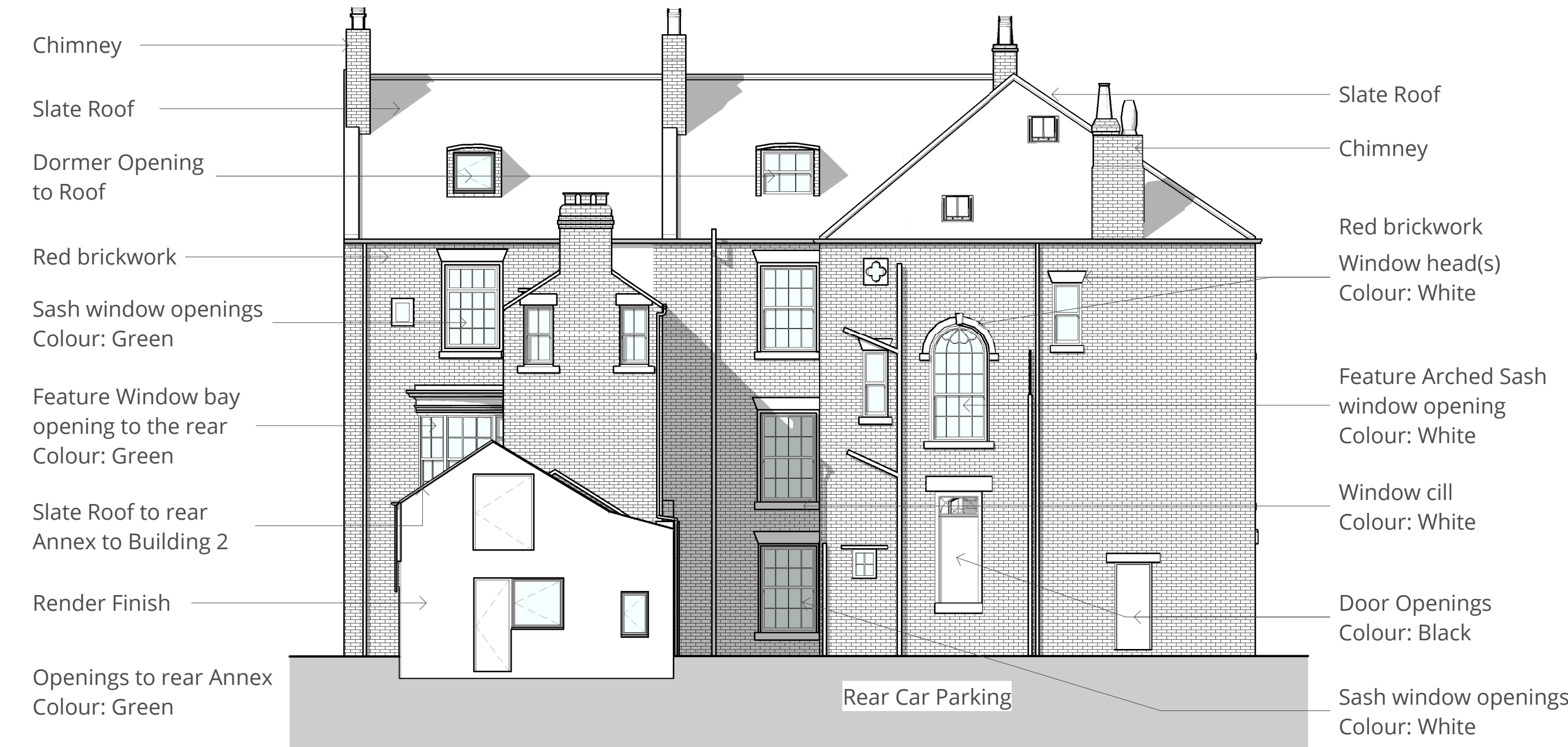
GA - Existing Rear Elevation 1 : 100
